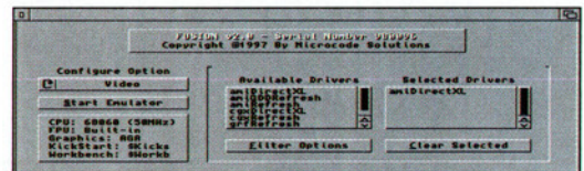
Fusion can access either an ATAPI or SCSI CD-ROM drive directly (top), needs contiguous memory (middle) and supports a variety of graphic drivers.
